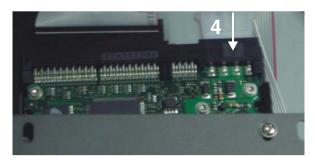
Fourth, connect the power supply to HDD  $\,$
